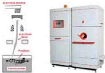
**Figure 1.** Arcam electron beam melting system (Arcam AB).
