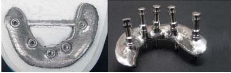
**Figure 3.** Milled titanium surface (left) and polished titanium surface (right).
