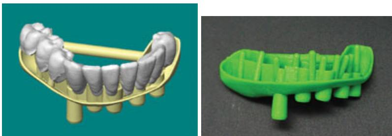
**Figures 10a and 10b.** Virtual model of planned prosthesis (a). Pattern for gold casting made using rapid prototyping (b).
